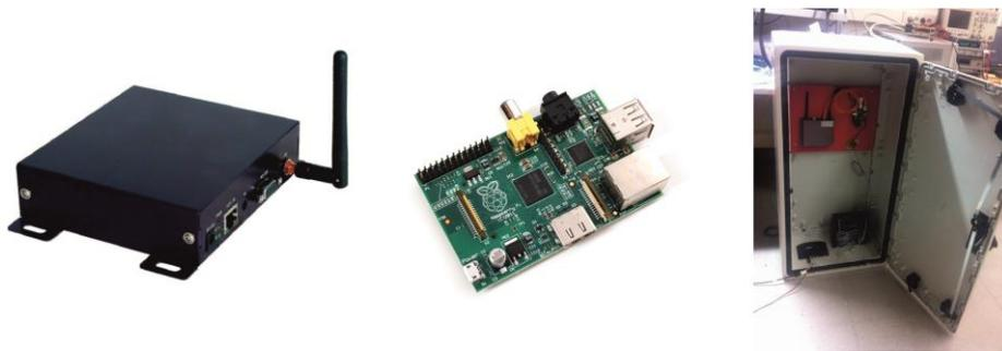
**Fig. 2.** MR3002A 2.4GHz RFID reader, raspberry Pi an prototype of the smart antenna.
