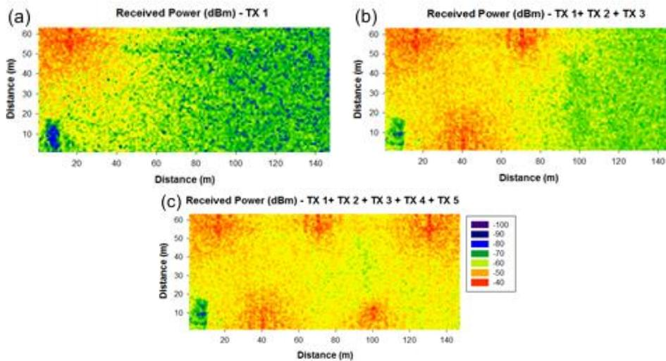
**Fig. 4.** RSSI 3D-ray simulation results obtained at a bidimensional plane at a height of 1m for different number of transmitters (a) TX 1 (b) TX1,TX2,TX3 (c) TX1,TX2,TX3,TX4,TX5.
