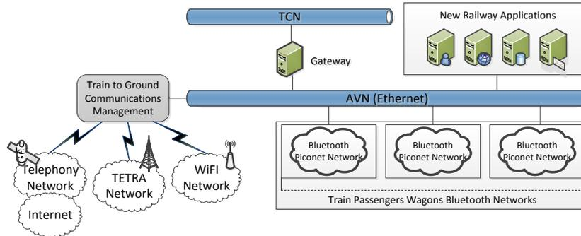
**Fig. 1.** Network architecture of the ubiquitous connected train
