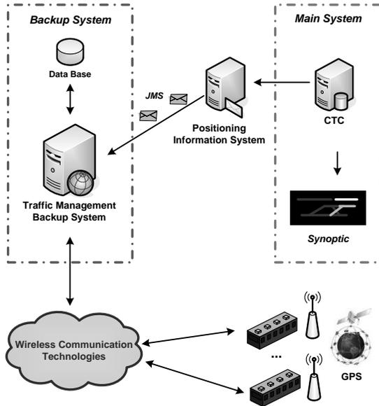
Fig. 4. Communication between the BTMS and the External Positioning Information System using Java Message Service (JMS).
