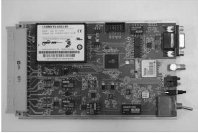
Fig. 3. On board hardware used to generate train positioning information by combining different on board positioning information sources (such as MEMS gyroscope, maps, ATP, odometer) and applying a logical approximation algorithm for matching railway lines and GPS coordinates.
