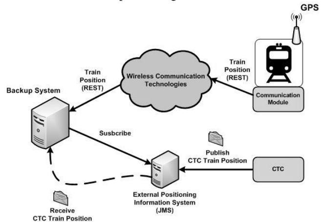
Fig. 2. Train positioning data reception in the BTMS, using a mixed distributed and centralized architecture.
