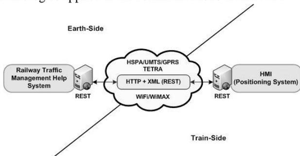
Fig. 5. 'Train-to-Earth' communications architecture.
