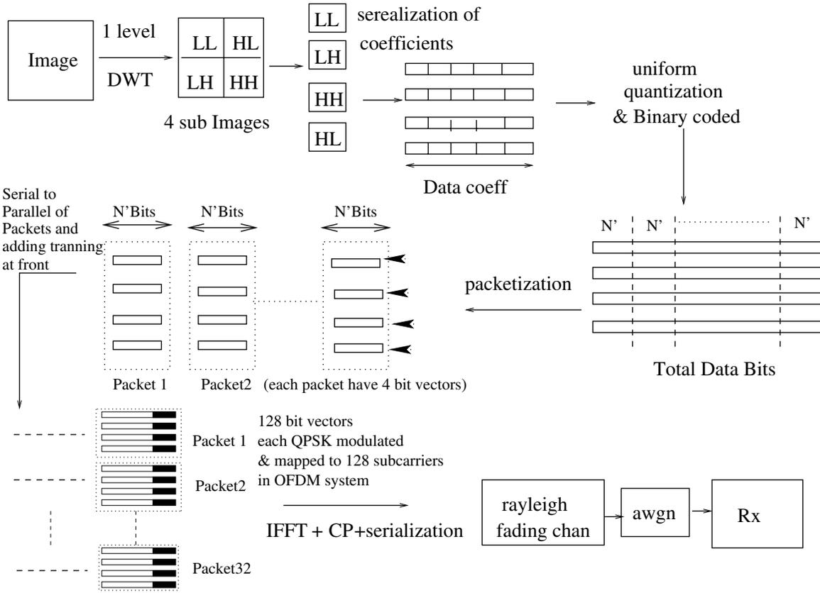
Fig. 1. DWT-OFDM system.
