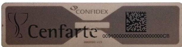
Figure 2. Confidex's Carrier Tough passive tag.
