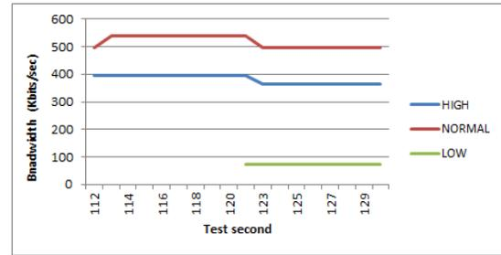
Figure 5. Low priority request launch and bandwidth reassignment
