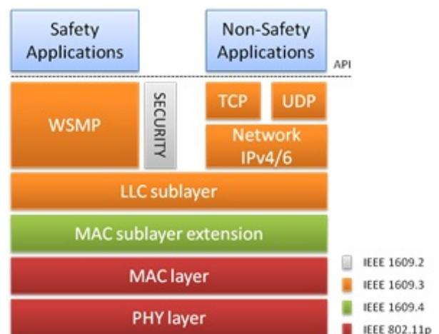
Fig. 1. IEEE WAVE/802.11p protocol stack
