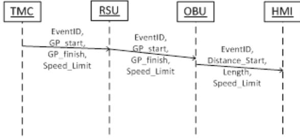
Fig. 3. Roadwork warning communication protocol
