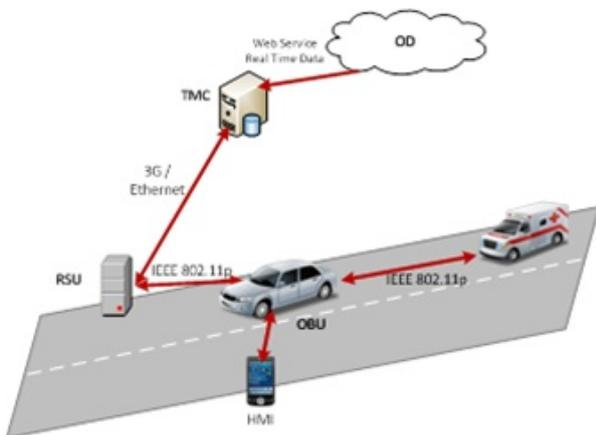
Fig. 4. Proposed platform of vehicular communications
