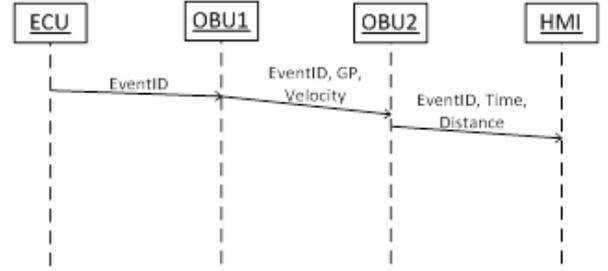
Fig. 2. Emergency vehicle warning communication protocol
