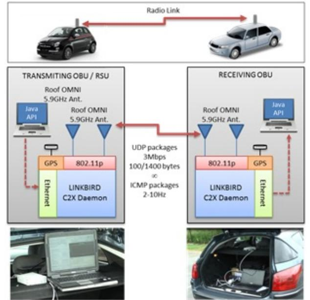
Fig. 5. On board hardware setup
