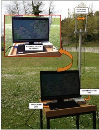
Fig. 6. RSU hardware setup
