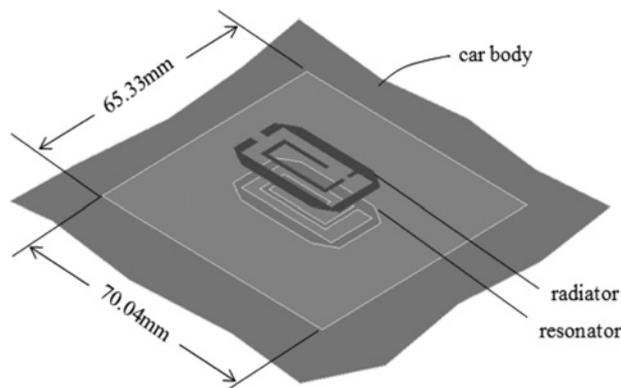
Fig. 6 Miniature antenna design printed onto the car body
