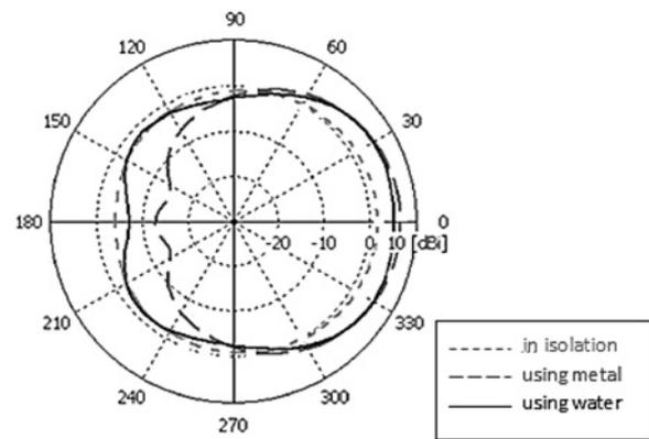
Fig. 4 Simulated radiation pattern of the tag
