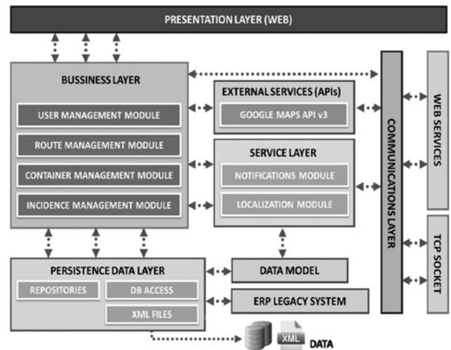
Fig. 10 Control software solution architecture
