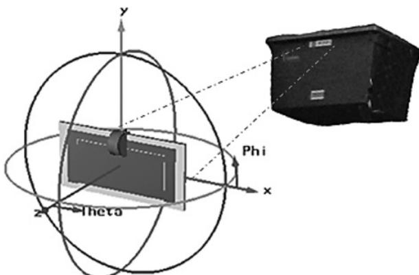
Fig. 3 RFID tag attached to the container
