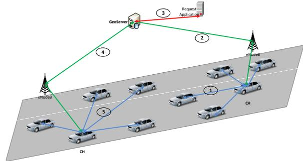
Fig. 1. Multi-technology information dissemination system:(1) Periodic broadcast of CAMs allows collecting information on the dynamic neighborhood relation. (2) Communication to geoserver of aggregated neighbor tables; (3) Data dissemination request and virtual infrastructure selection at geoserver; (4) Information dissemination execution and (5) Local data dissemination by virtual infrastructure.
