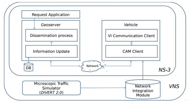
Fig. 2. Demo simulation platform: The architecture and algorithm is implemented in the NS-3 discrete network simulator, which mimics the behavior and the interaction between Vehicles and the Geoserver. The realistic mobility of vehicles is generated by DIVERT 2.0. The Network Integration Module (NIM) enables the bidirectional interaction between network and traffic simulators.
